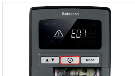
VISIBLE AND AUDIBLE COUNTERFEIT BANKNOTE ALARM
