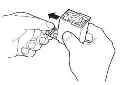
(2) If a staple sheet is come out of the cartridge, push it into the cartridge. It could cause a jammed staple.
