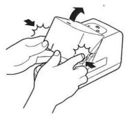
(2) Load the staple cartridge in the arrow direction.
