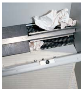
Automatic mechanical feeding system with revolving flaps
