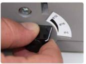
The depth gauge feature allows the operator to adjust the punched hole margin from 2 mm to 4,5 mm. This adds strength to the bound edge.
