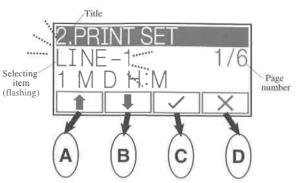
Functions of operation keys (A - D) are displayed by the icons on  $LCD_\alpha$  You can operate flashing item by clicking down the corresponding keys.
