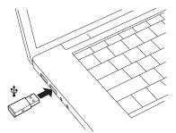
The USB adapter LED is solid red when inserted and then turns solid blue to indicate the headset is connected to the USB adapter. If you are wearing your headset you will hear "Base connected" to indicate the connection has been established. When on a call, the LED on the USB adapter flashes blue. When not on a call the LED is solid blue.
